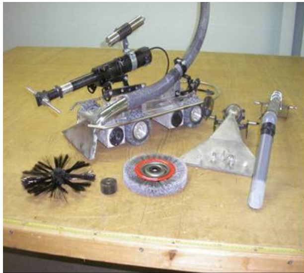
Fig. 2. Remote-controlled tool carrier equipped for intervention inside the ventilation duct
