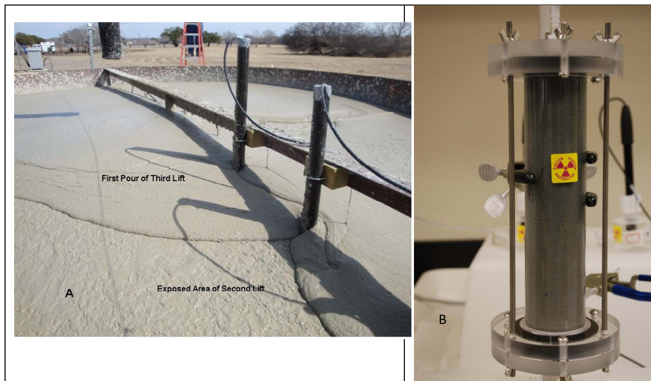
Fig. 5 (A) Grout Monolith and (B) Column Experiments Conducted at CNWRA in San Antonio, TX, with Cementitious Grout Materials proposed for WIR applications.
