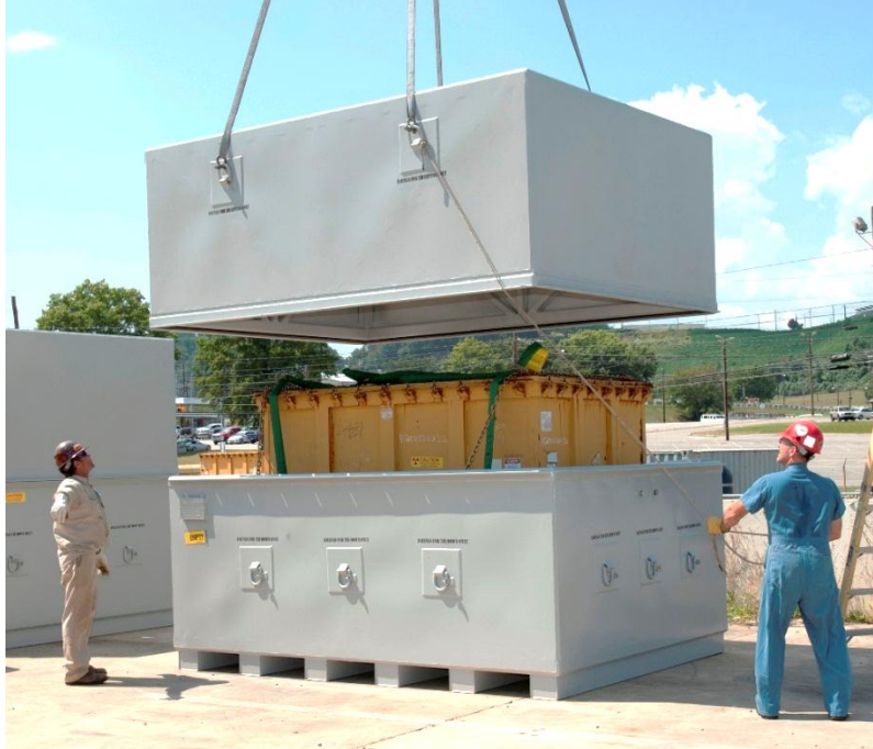
Fig. 7. Lowering the lid during overpacking the salt bath and legacy box.
