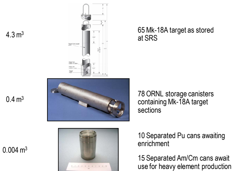
Fig. 5. Processing Mk-18A targets to oxide powders reduces shielded storage requirements by three orders of magnitude.
