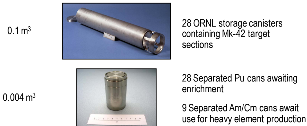
Fig. 6. Processing Mk-42 targets to oxide powders reduce shielding storage requirements by a factor of 25.
