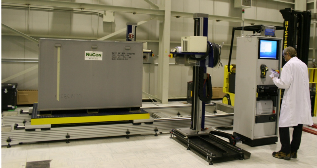
Figure 1. B-1000 container and Waste Assay System (Box Counter)
