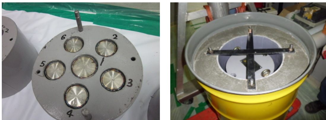
Fig. 3. Lead Shield and Concrete Lining Drum
