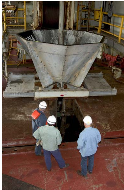
Fig. 3. Re-entry Cone Assembly Staging in Moonpool [13].
