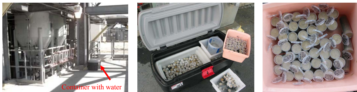
Figure 2. Curing container in Z-Area and samples with open lids arranged in the container.
