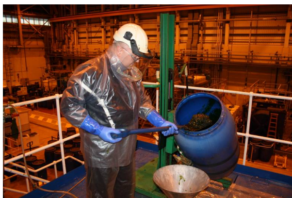
Fig 7. Loading a corrosive residue into a leach vessel.
