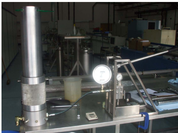
Figure 5- Collapse test rig set up
