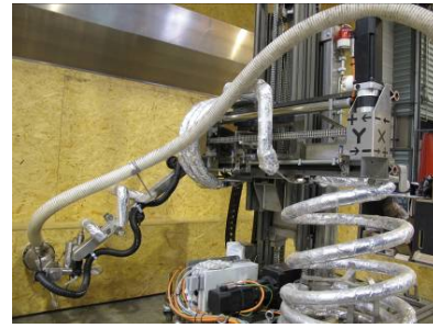
Figure 10 : Installation of HP hoses on the carrier
