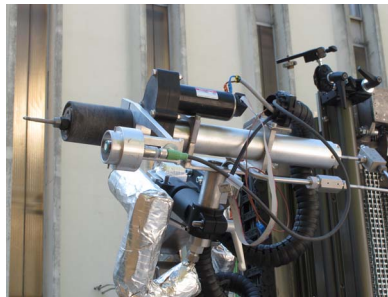
Figure 17 : The new lancing onto the automatic carrier
