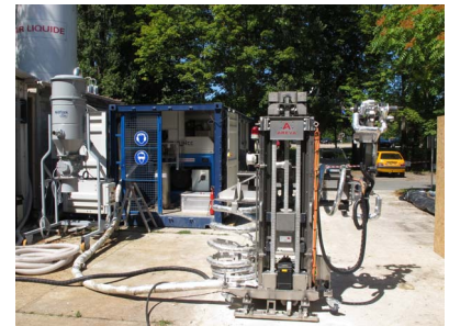
Figure 18 : The NiThrow™ solution (carrier; skid, vacuum system, tank)
