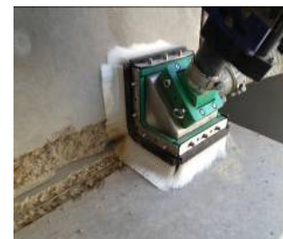
Figure 8 : Shroud system for internal angular surface
