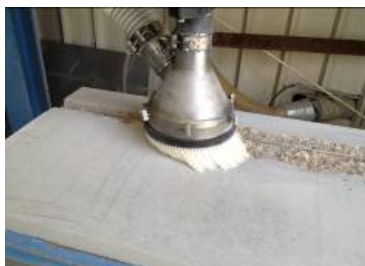
Figure 6 : Shroud system for flat surface
