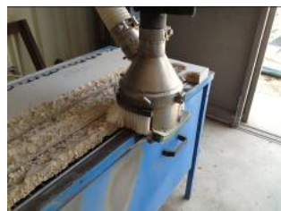
Figure 7 : Shroud system for external angular surface
