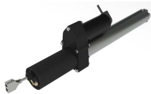
Figure 2 : CAD picture of the new lancing tool
