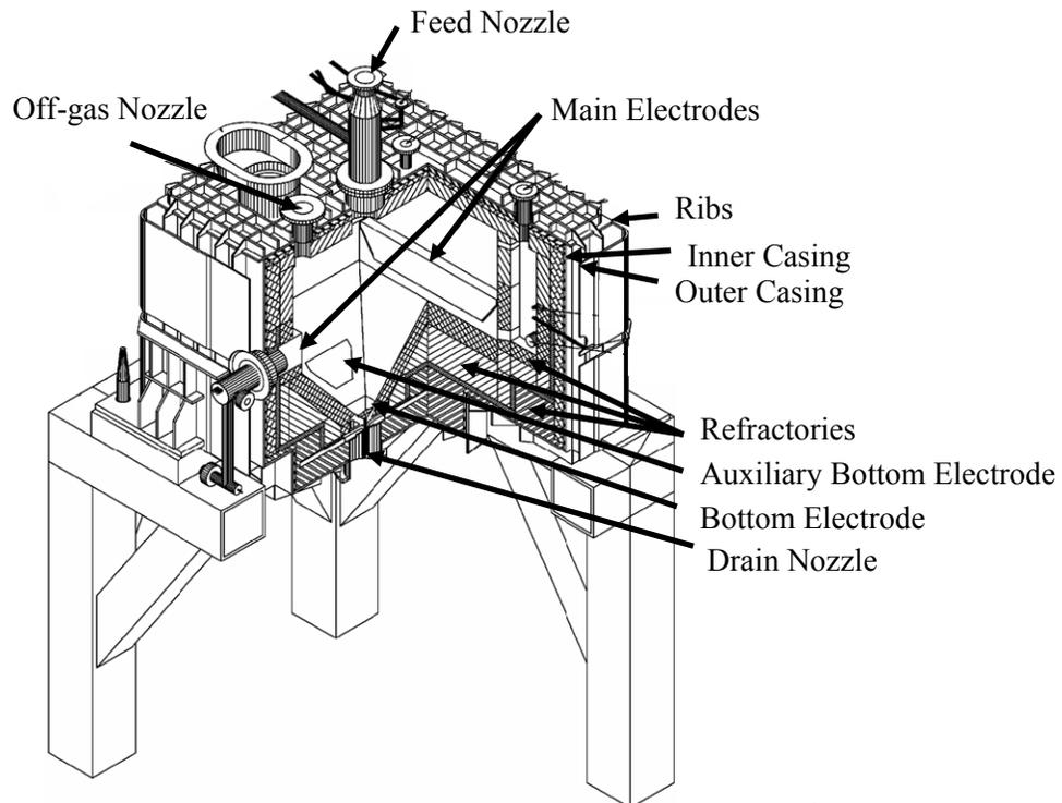
Figure 1: The Glass Melter (Liquid-Fed Ceramic Melter) <sup>1</sup>
