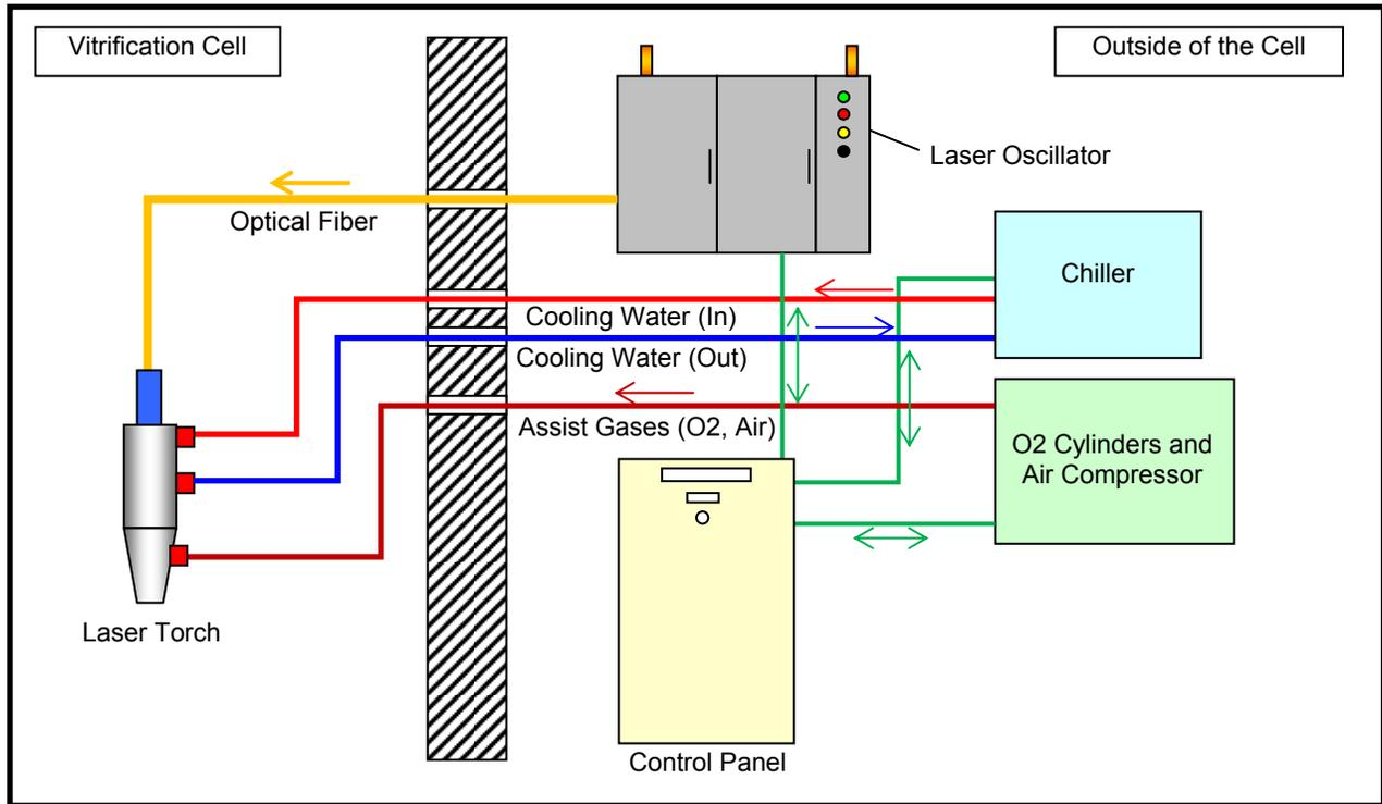
Figure 4: Overview of remote fiber laser cutting system
