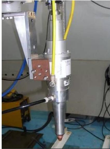
Figure 5: Laser Torch (used for cutting test)
