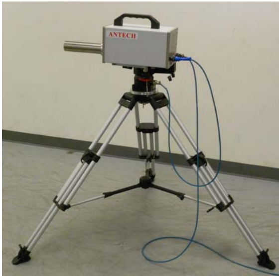
Figure 1. RadSearch detector head and pan and tilt unit mounted on a tripod for measurement. The collimator barrel is fitted.
