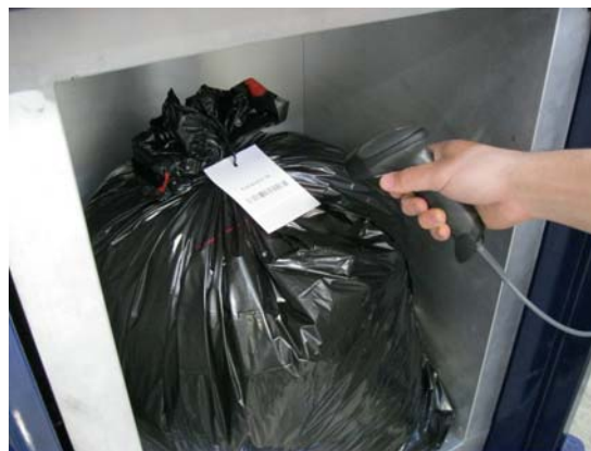
Figure 2. Interior of the measurement chamber of the Model G3301-200 Waste Segregation and Clearance Monitor showing the bar code of a waste bag being recorded.
