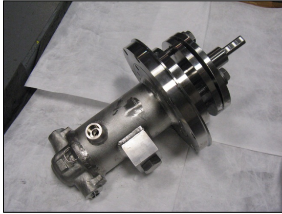
Figure 7: 1/2" EBV at Final Inspection
