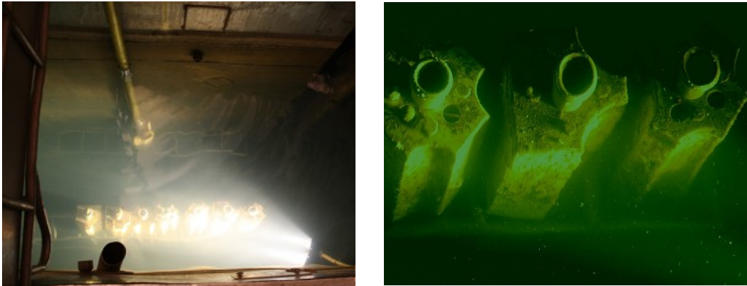
Fig. 1. Beryllium blocks stored in the storage pool in the central MR hall.
