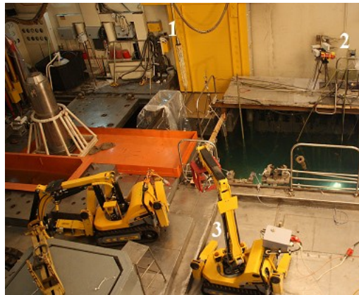
Fig. 2. Positioning of measuring equipment during beryllium blocks' characterization: 1 – Dosimeter; 2 – “Gammavisor”; 3 – “Gamma-Pioneer”.
