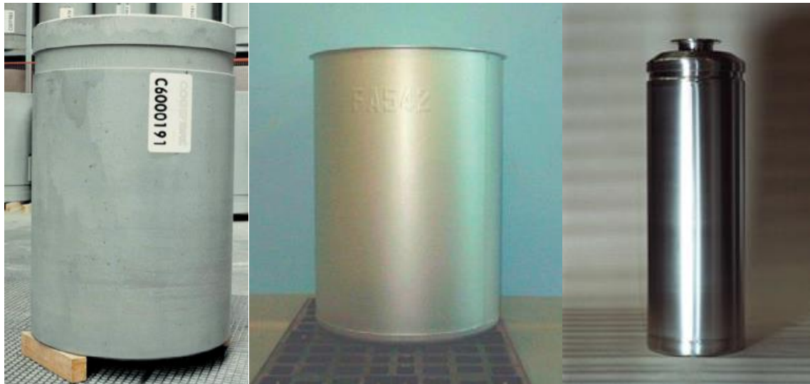
Fig. 1. Example of intermediate level waste packages (a) solid maintenance waste in fiber reinforced concrete containers (CBFC'2), (b) bituminous waste package from effluent treatment, and (c) compacted waste packages CSD-C).
