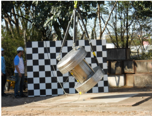
Figure 6. Second 9 m drop test – 51°, lid down
