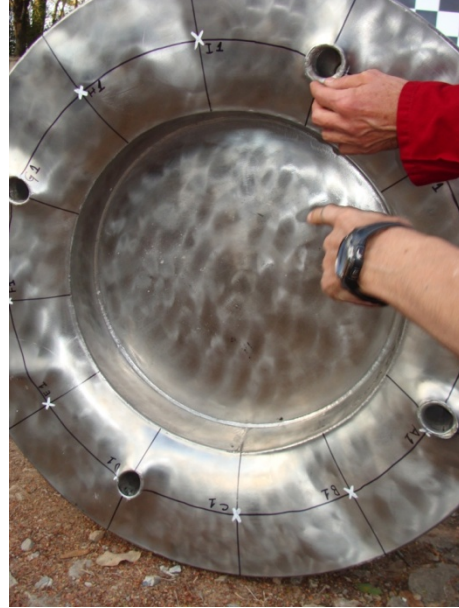
(b) Small damages on the impacted shock absorber
