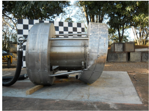
Figure 6. Second 9 m drop test – 51°, lid down
