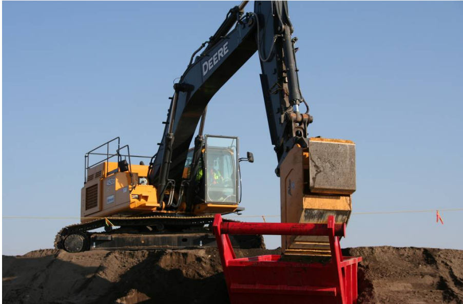
Figure 4. Crushing and mixing test bottles with grout within a mix box.
