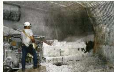
SALT WALLS A continuous miner is used to carve disposal rooms out of the salt formation, nearly a half-mile below the surface.
