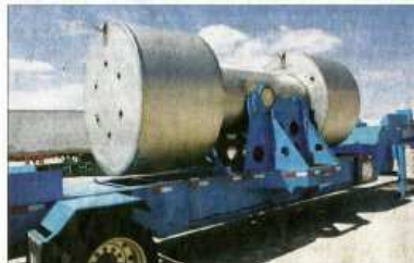
TRANSPORTING WASTE A container called RH-72B is a lead-lined cask used for shipping remote-handled transuranic waste.
