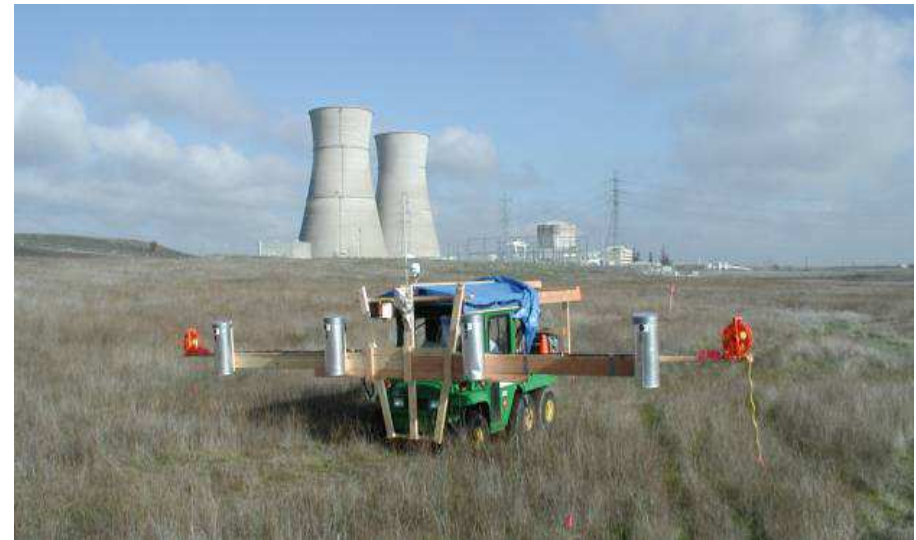
Shonka Research Associates - Subsurface Multi-Spectral Contamination Monitor (SMCM) at Rancho Seco
