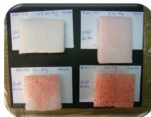
Baseline with commercial glycerin fog. Test coupons show lack of penetration (visible beading) and inconsistent coverage.
