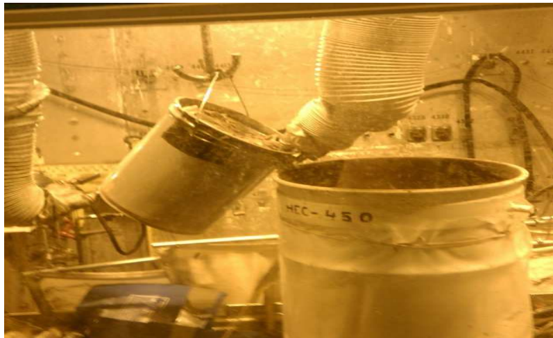
Scrubber Vessel Solids Removal and Packaging (SBS)
