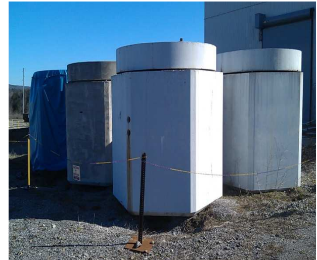
Spent Fuel Resins Packaged in Poly High Integrity Containers (HICs) Stored in Concrete SUREPAKS
