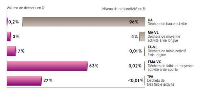
The level of radioactivity and the radioactive period of the HL and ILL wastes do not allow them to be securely stored in surface or shallow depth storages.
