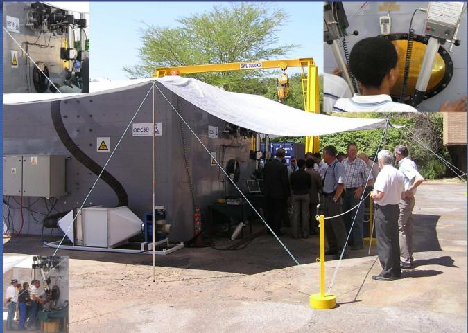
Mobile Hot Cell – used to remove and condition high activity sources in devices
