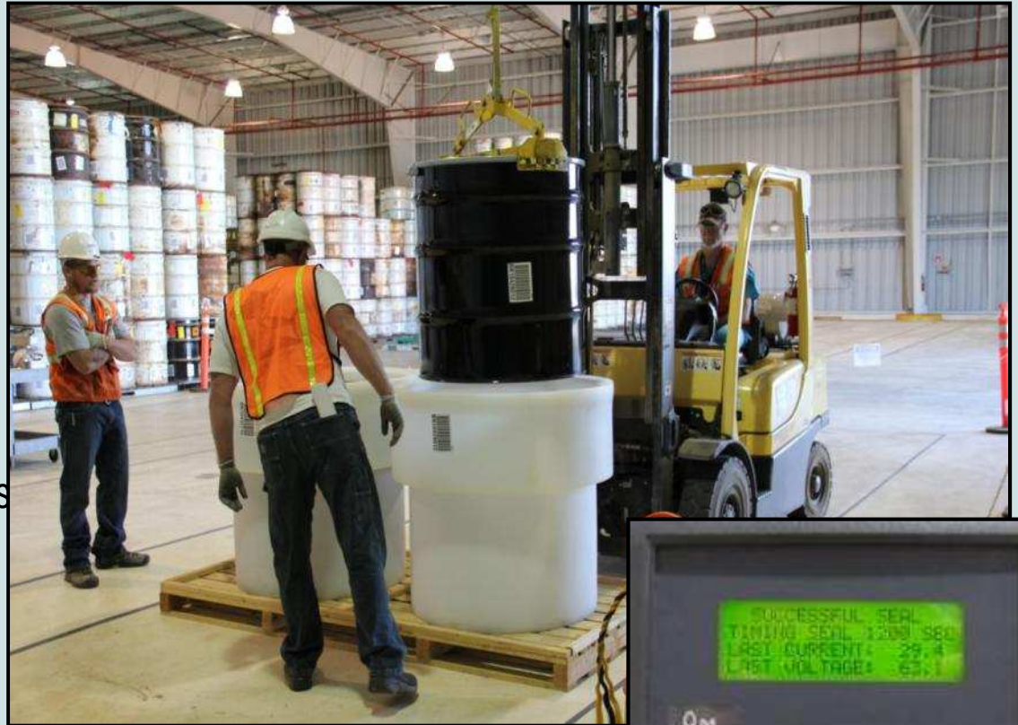
A product drum containing Mixed Low-Level Waste is lowered into a high density polyethylene “macro-pack.” The lid of the macro-pack contains heating wires. An electric current is sent through the wires to permanently seal the container.
