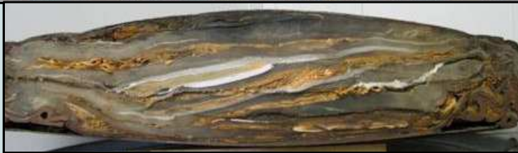
55-gallon drum post Supercompactor = a puck
