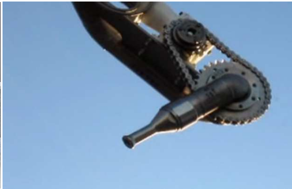
Enhanced Reach Sluicing
