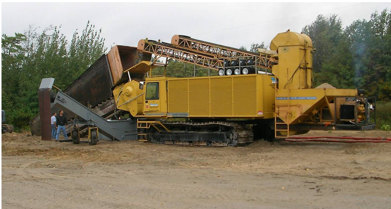
Fig.2. One-pass trencher used in installation of the PTW.
