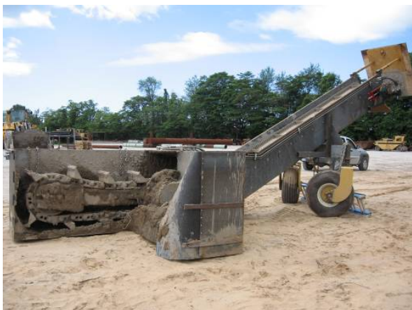
Fig.4. One-pass trencher soil conveyor.
