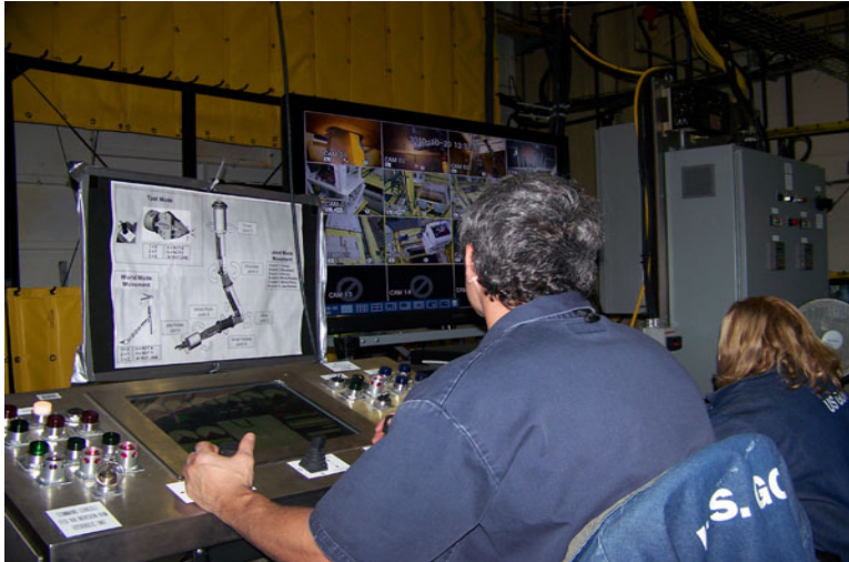
Figure 3: Operators inside the XC-1 command center monitor operations inside XC-1 and the XCR using the camera system installed inside and outside the cell. The command station for the robotic arm is in front of the operator seated at left.
