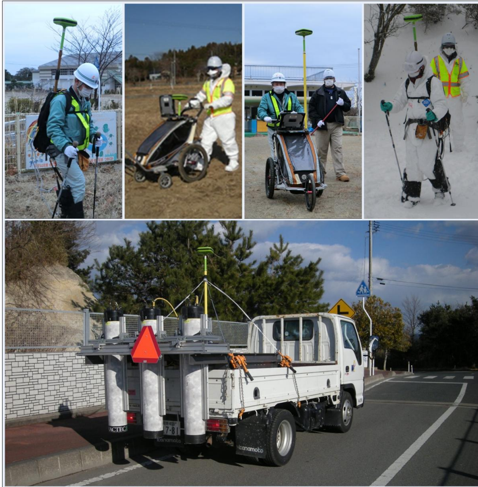
Figure 2. ScanPlot SM Systems Used to Characterize Contaminated Land in Hirono Town and Naraha Town
