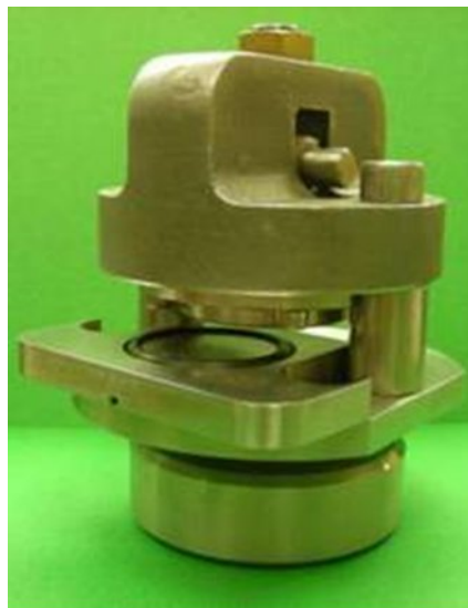
Figure 3. Compression Stress-Relaxation (CSR) Fixture – Shawbury/Wallace C16
