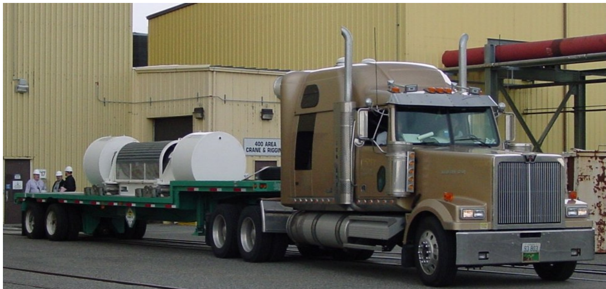
Fig 2. The T-3, with an inner container, being used to ship Fast Flux Test Facility sodium bonded fuel.
