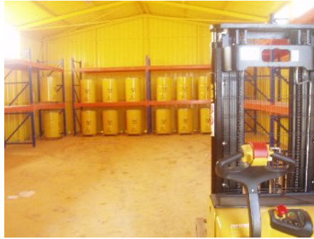
Fig 3. Waste packages (200 L) in interim storage.
