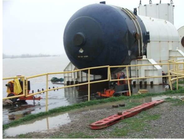
Figure 2. Barge transport of a steam generator
