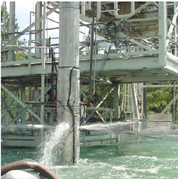
Fig 6. Pump testing. All pumps designed and procured for waste tank usage were rigorously tested in a full scale test facility.
