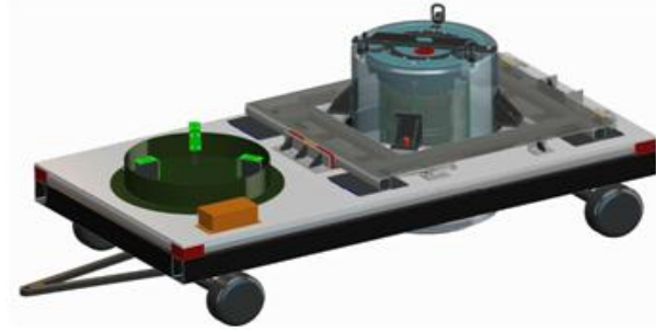
Fig.1. FCS: Trailer with shielding cask, mounted on movable platform
