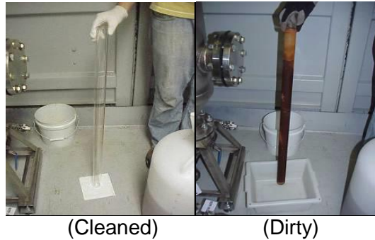
Figure 2. Fouling of the UV Light Apparatus
