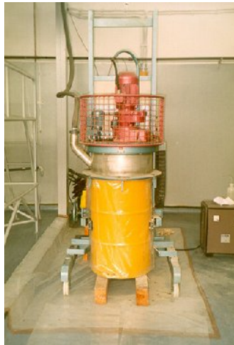
Fig 4. In-drum mixer for cementation process.
