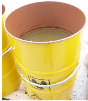
Fig 3. Radioactive sludge in drum.
