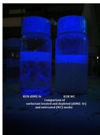
Figure 7.a) Qualitative determination of media oil uptake by fluorescence b) quantitative determination of surfactant retention of oil by the indirect removal of Tc 99.
