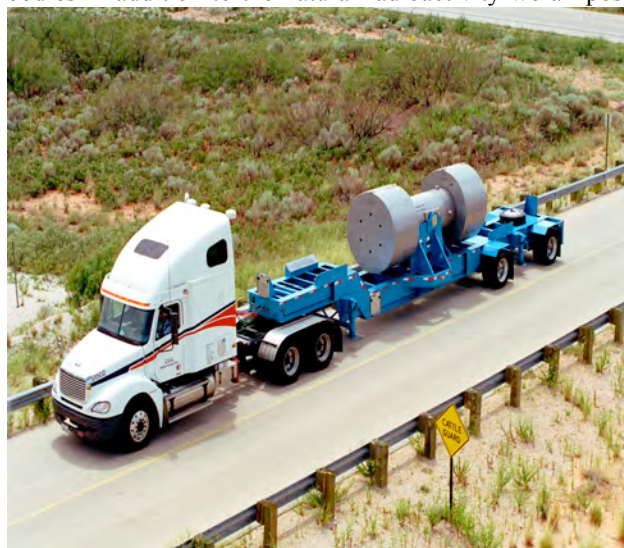
Fig. 4. High-activity remote handled nuclear waste, some of it from reprocessing of spent fuel from old weapons reactors, being transported to the WIPP site in New Mexico in a 72B cask. 10,000 shipments of nuclear waste to WIPP has never resulted in any release or harm to humans or the environment.
