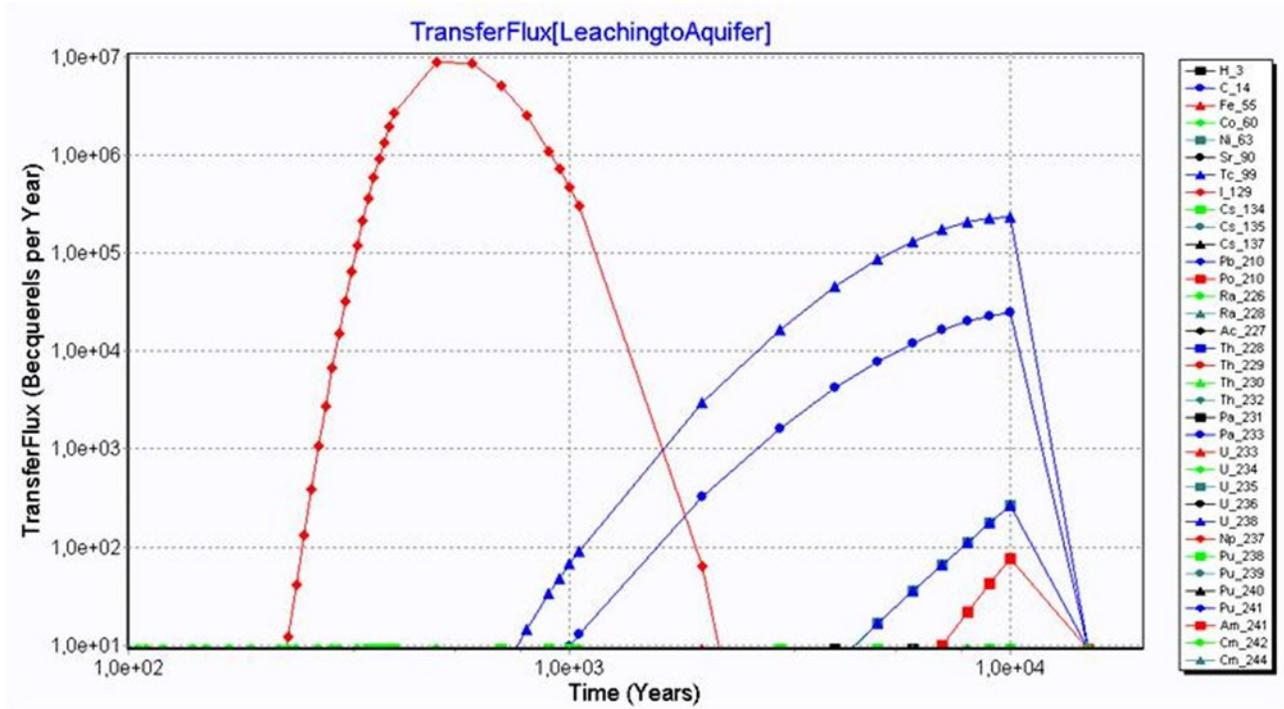
Fig. 3. Radionuclide flux from the unsaturated zone to the saturated zone.
