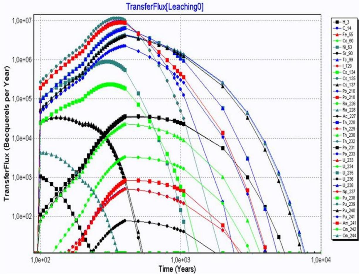
Fig. 2. Radionuclide flux from the repository to the unsaturated zone.
