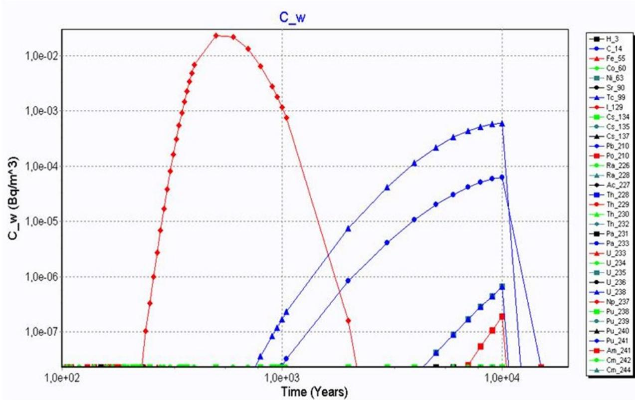
Fig. 4. Concentration of key radionuclides in the well water.
