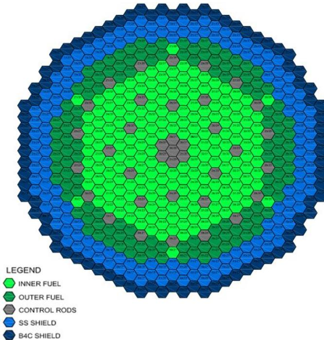
Fig 1. Radial view of the ARR burner design
