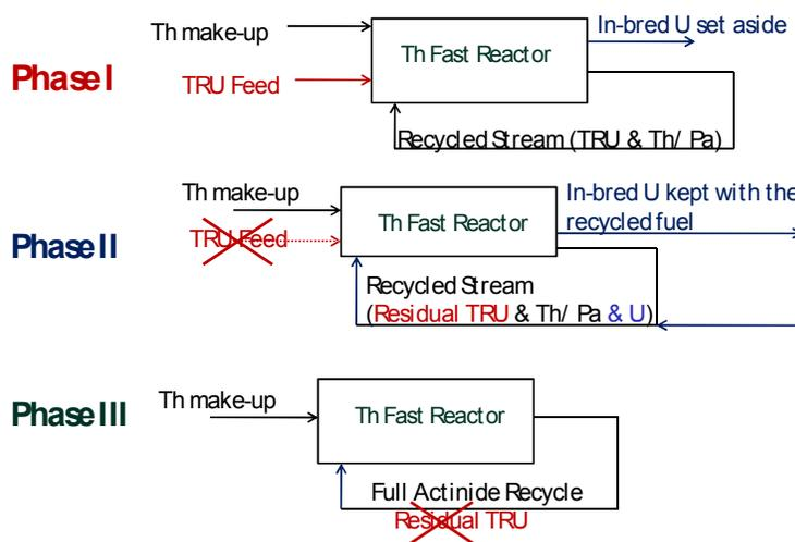
Fig 4. Schematic depiction of the 3-phase simulation to transition from TRU burning to closed Th-cycle
