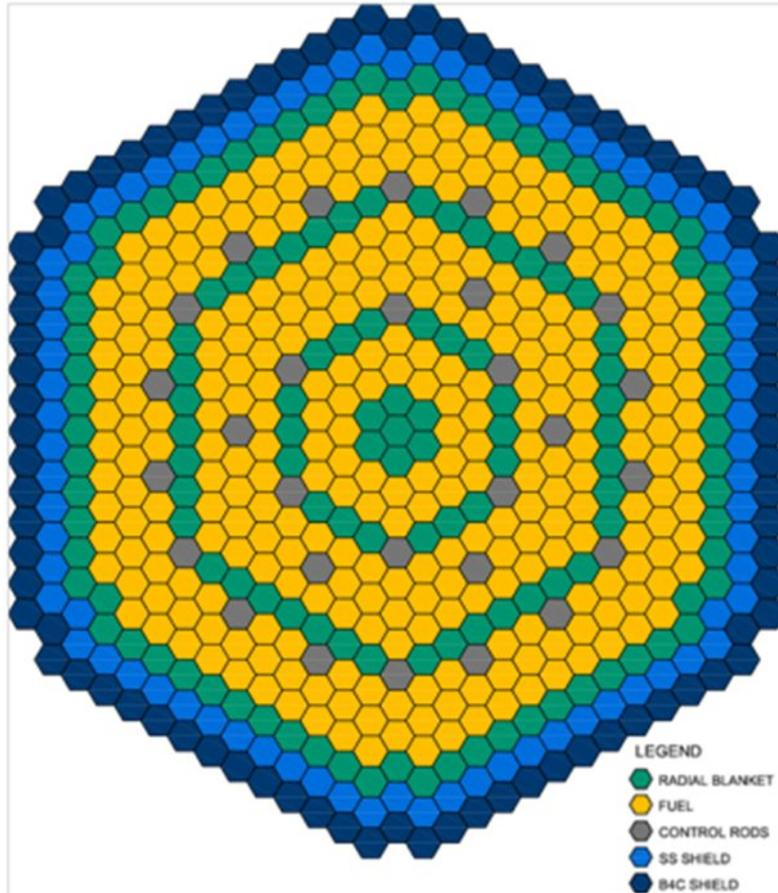
Fig 3. Radial view of the heterogeneous ARR breeder design
