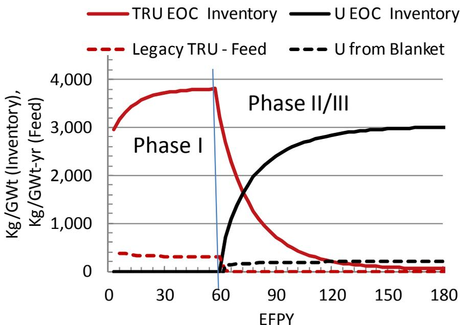
Fig 5. Trend in TRU and U core inventory and feed requirements from TRU burning to closed Th-cycle
