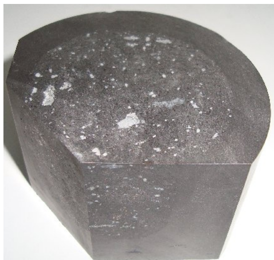
Figure 8: IGM sample with virgin Magnox graphite mixed with mineral and metallic scrap
