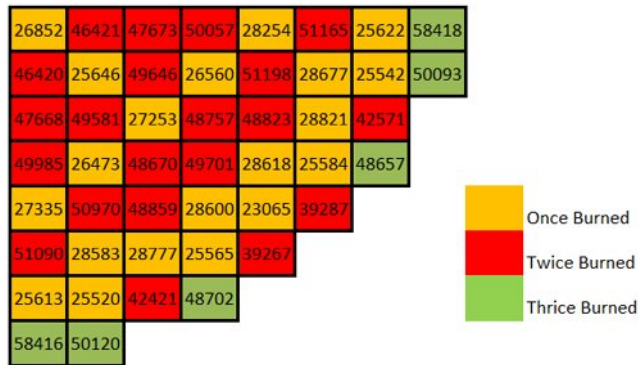
Figure 2. Radial Burnup at End of Cycle (22000 MWD/MTM)
