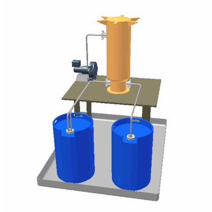
Figure 2 Example of Model of a Process Module (Module B5 - Simple Filtration)
