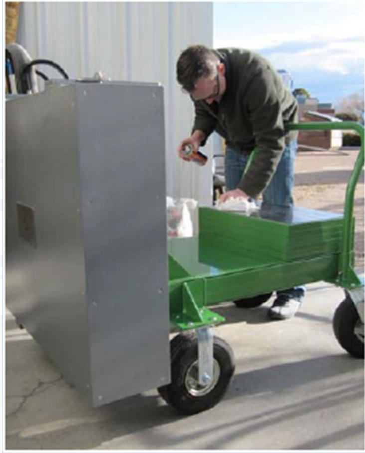
Figure 3. 618-10 Burial Ground Drum Radiation Screening Tool
