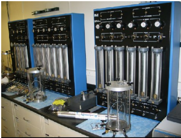
Figure 5. Hydraulic conductivity test apparatus
