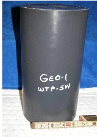
**Fig. 3. Clay Based 15¼ cm x 30½ cm GEO-1 Monolith for ESTD WTP-SW at 68% FBSR Loading.**
