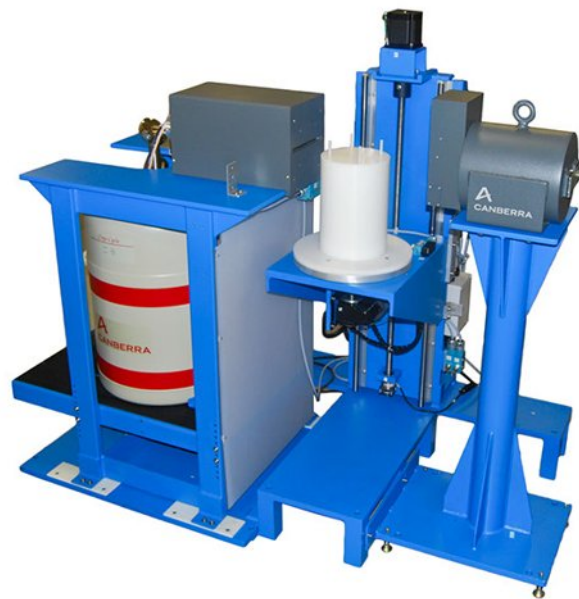
Figure 1. Photograph of the Can SGS as built in 2011 at Canberra's Meriden Facility.
